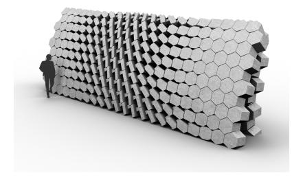
We began with some studies, using simulation, of the relation between the form and openness of a notional wall and the resulting wind performance and/or air pressure around the wall. While formal variation produced somewhat predictable results it was the relationship between openness and air-pressure which began to fascinate us most.
